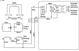
Figure 31 - Wiring Diagram, Models RGH3000 and RGH3000PR
